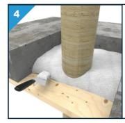
When the desired consistency has been reached, apply the Multimortar with a trowel or pump, and make sure that it runs into all corners and around the service penetration. Firmly push the mortar into the gap to eliminate any air bubbles.
