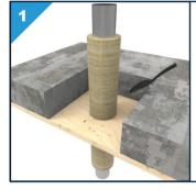
Make sure that the service penetration and the gap are free from dust, dirt and grease. Wet the gap with water for better adhesion.
